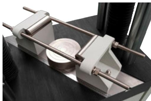
Bending testing device
