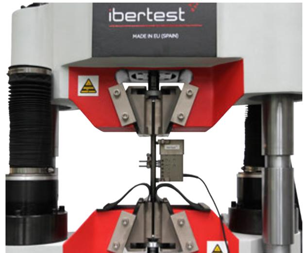
Tensile test of a cylindrical specimen. Deformation measurement through clamp extensometer IB-MFA20
