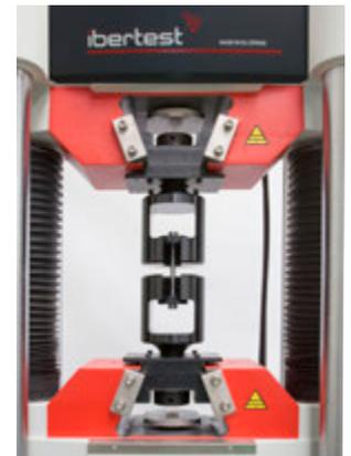
Accessory: tensile device for cabezales for button or/and threaded shouldered metallic specimens
