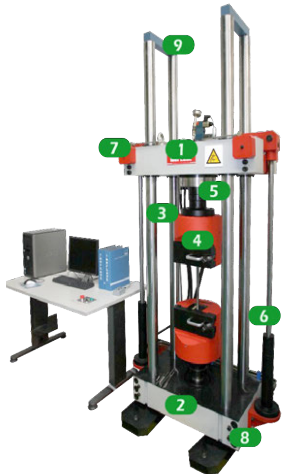
UMIB-600, with actuator fixed under the lower crosshead
