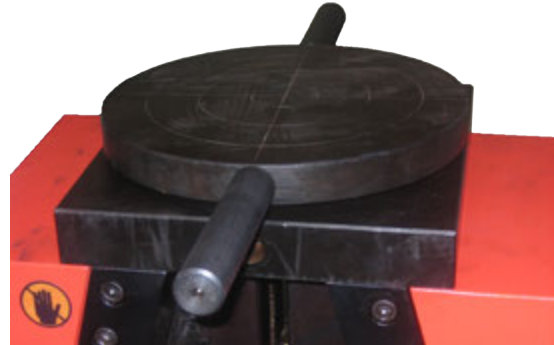
Compression plate mounted on hydraulic grip
