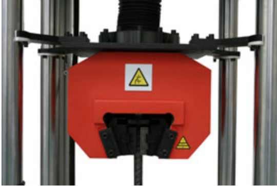
Hydraulic tensile gripping heads
