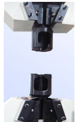
Tensile of headed specimens
