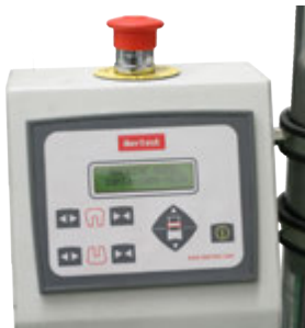
Remote Control for opening / closing jaws and piston positioning
