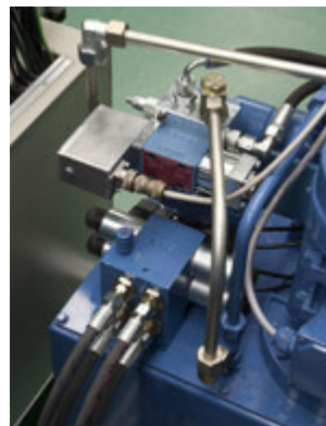
Hydraulic group, inside of the control desk
