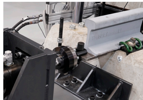
Longitudinal rail restraint test set-up
