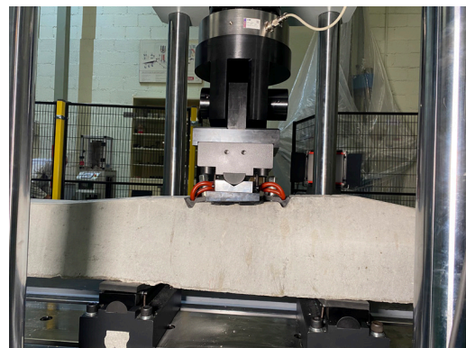
View of a sleeper during the under-rail section fatigue test
