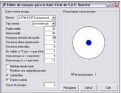
Cement consistency as per ASTM C-187
