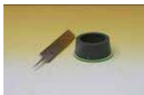
Mould, glass and sliding weight with conical needle for gypsum as per EN 13.279-3.
