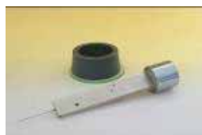
Mould, glass and sliding weight with needle and counterweight for additives as per EN 480-2
