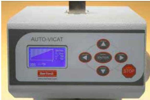
Detail of the front panel with 6-keys sensitive keyboard and graphic screen.
