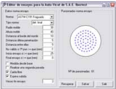
Cement setting as per ASTM C-191
