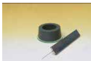
Mould, glass and sliding weight with needle as per ASTM C191
