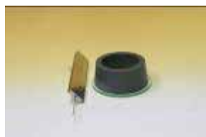
Mould, glass and sliding weight with needle as per EN-196-3.
