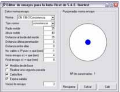
Cement consistency as per EN 196-3
