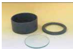
Mould, glass and sliding weight with needle as per EN-196-3.
